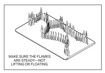
Figure 35. Burner Flame Patterns
